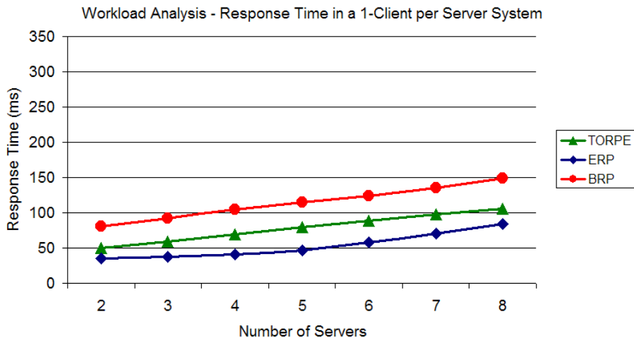
Figure 4.15: Response time of the replication protocols for a submission rate of 10 TPS varying the number of servers
