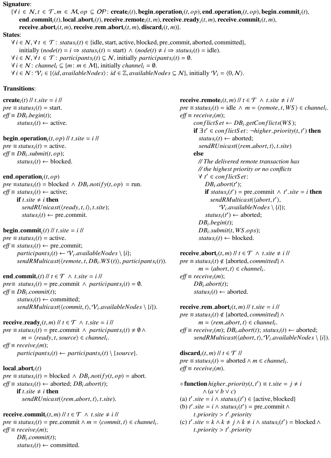
Figure 3.2: State transition system for the Basic Replication Protocol (BRP). pre indicates precondition and eff effects respectively
