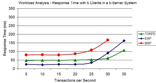
Fig. 4. Response time of the replication protocols varying the submission rate
